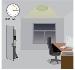
After heat leaves the area, the sensor will keep light 100% ON for a hold-time period, then turn OFF light automatically.
