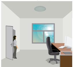
With enough ambient brightness, sensor will keep the light OFF even though it detects heat.
