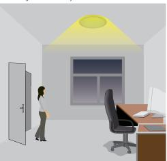
When ambient brightness gets lower than the preset daylight lux level, the sensor will turn ON light once it detects heat in the area.
